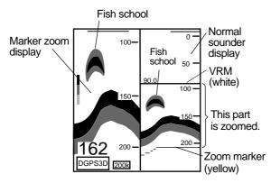
Figure 2-7 Marker-zoom display plus normal sounder display
